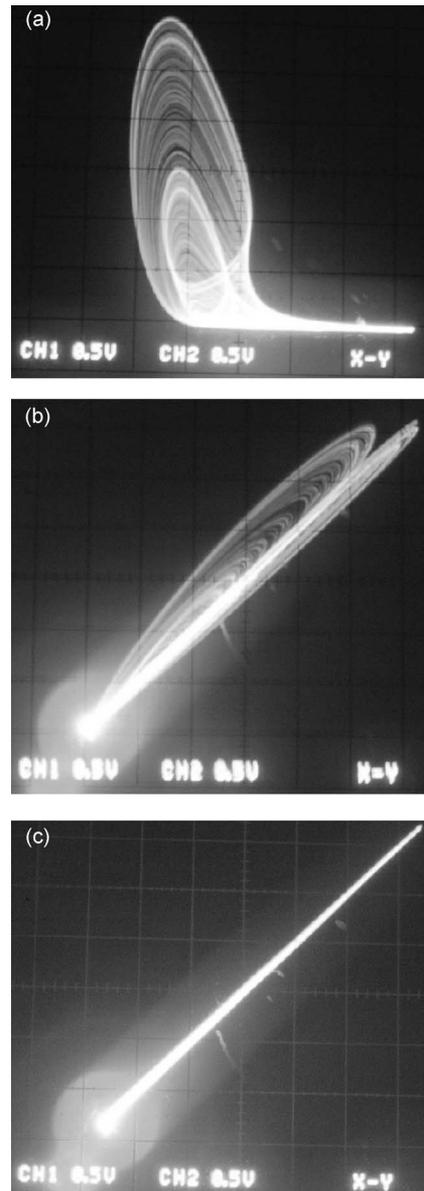
FIG. 10. (a) The chaotic attractor of the LC oscillator,  $v_c$  vs  $v_F$ . (b) and (c) The synchronization manifold  $v_F$  vs  $v'_F$ . (b) The response system with feedback coupling but without parameter mismatch compensator. (c) The response system with both feedback coupling and parameter mismatch compensator.
