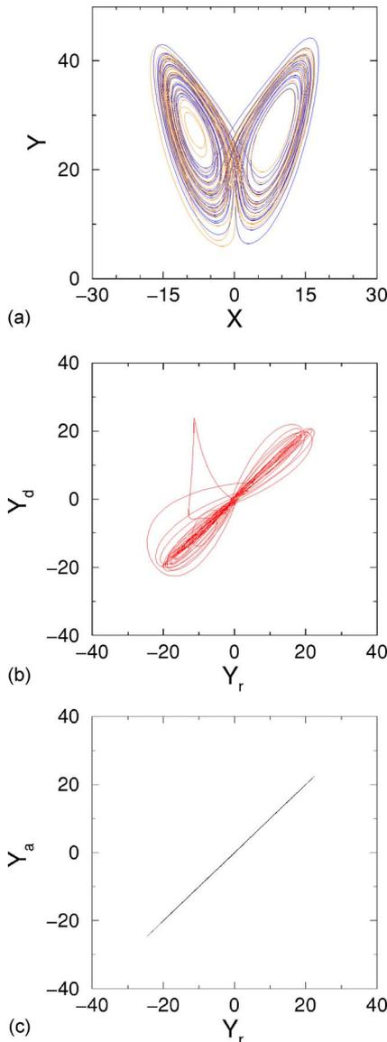
FIG. 4. GS rather than CS observed between two identical systems with generalized feedback coupling.  $\epsilon=3$ . (a) The attractors in the drive (black), response, and auxiliary systems (gray; they are totally overlapping). (b)  $y_d$  vs  $y_r$ . (c)  $y_a$  vs  $y_r$ .
