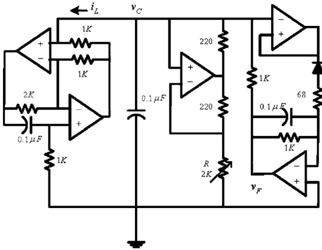
FIG. 9. The electronic circuit of the LC oscillator.
