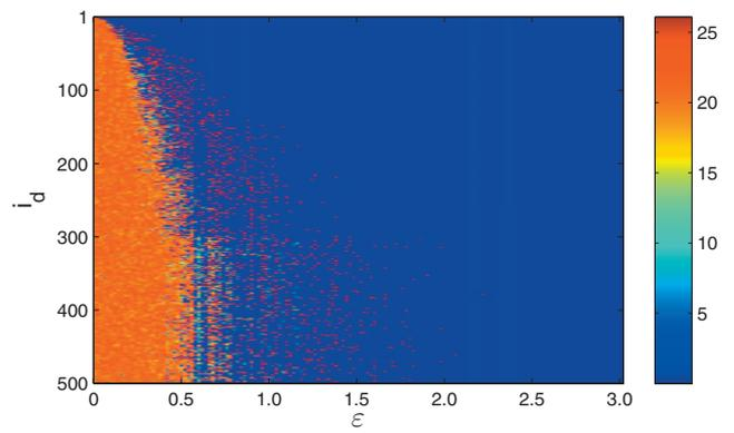
FIG. 4. (Color) Color map of  $d(\epsilon, i_d)$  in the two-dimensional parameter space  $(\epsilon, i)$ , characterizing the development of GS for 500 nonidentical Lorenz chaotic oscillators on a scale-free network. The network is the BA model with  $m_0=m=3$  (Ref. 21). The development of GS in the network is similar to the situation shown in Fig. 1.
