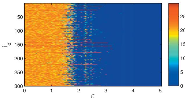
FIG. 9. (Color) Color map of  $d(\epsilon, i_d)$  in the two-dimensional parameter space  $(\epsilon, i)$ , characterizing 300 hybrid Lorenz chaotic oscillators on a scale-free network. The network is the BA model with  $m_0=m=3$  (Ref. 21).
