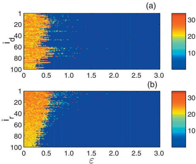
FIG. 5. (Color) Color maps of  $d(\epsilon, i_d)$  and  $d(\epsilon, i_r)$  in the two-dimensional parameter space  $(\epsilon, i)$  for nonidentical Lorenz oscillators on a regular network. The network has 100 nodes, and each node has six nearest neighboring connections.
