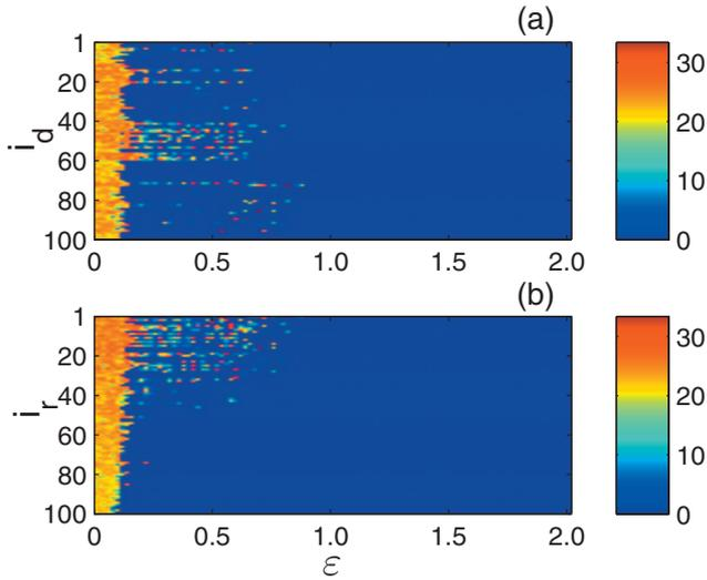
FIG. 7. (Color) Color maps of  $d(\epsilon, i_d)$  and  $d(\epsilon, i_r)$  in the two-dimensional parameter space  $(\epsilon, i)$  for nonidentical Lorenz oscillators on a clustered network. The network has 100 nodes which are evenly divided into five modules. Nodes within each module are fully connected. Any two nodes in different modules have probability  $\rho=0.005$  to connect each other.
