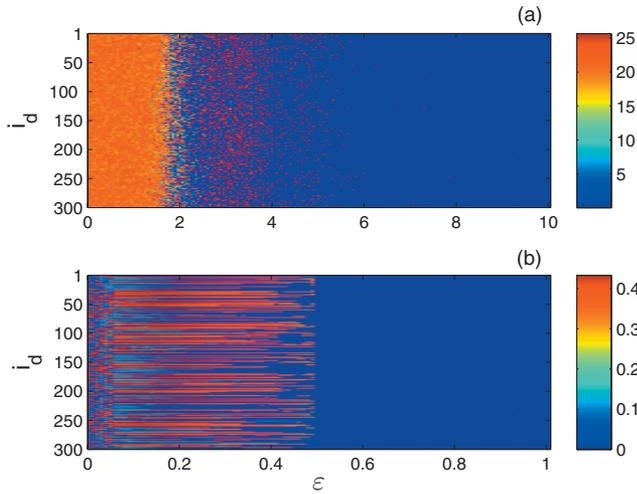
FIG. 8. (Color) Color maps of  $d(\epsilon, i_d)$  in the two-dimensional parameter space  $(\epsilon, i)$ , characterizing the development of GS for 300 identical Lorenz chaotic oscillators (a) and 300 identical Logistic maps (b) on a scale-free network. The network is the same as in Fig. 1. Compared with Fig. 1, the effect caused by the normalized coupling strategy is obvious.
