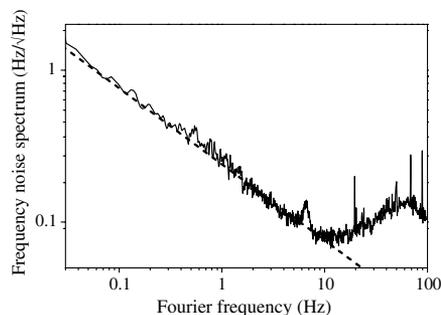
Fig. 6. Frequency noise spectrum of one cavity-stabilized laser system. The dashed line shows the calculated thermal-noise-limited frequency noise spectrum of one cavity at  $0.24 \text{ Hz}/\sqrt{f}$ .
