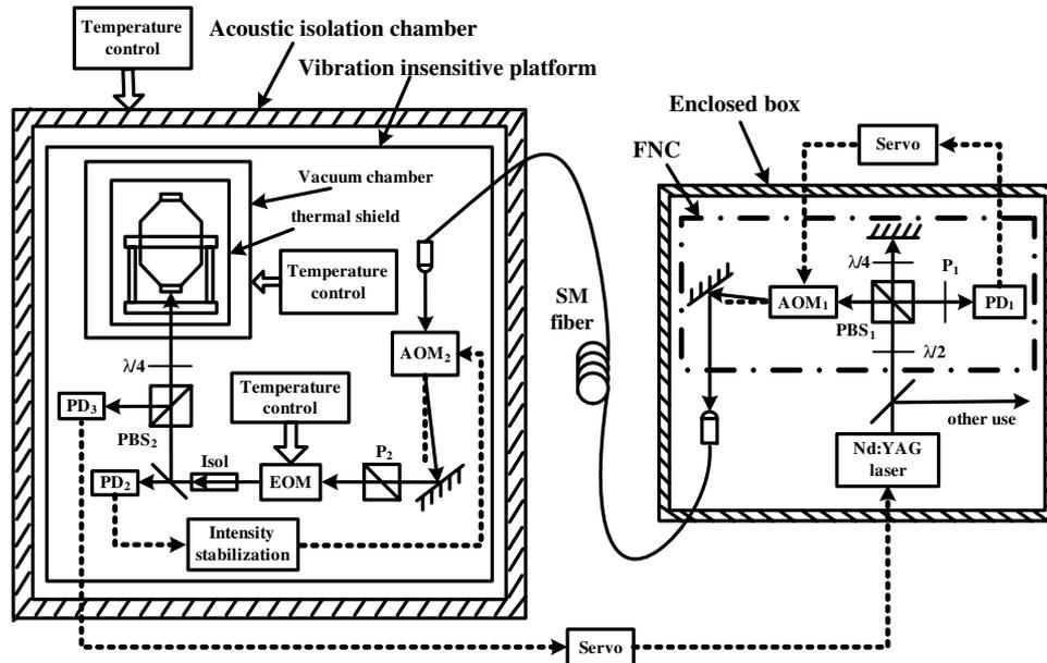
Fig. 1. Schematic diagram of the experimental setup for Nd:YAG laser frequency stabilization. AOM, acousto-optic modulator;  $P$ , polarizer; EOM, electro-optic modulator; Isol, optical isolator; PD, photodetector; PBS, polarization beam splitter;  $\lambda/4$ , quarter-wave plate;  $\lambda/2$ , half-wave plate; FNC, fiber noise cancellation; SM, single-mode.
