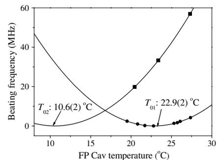
Fig. 2. Measurements of the zero-expansion temperatures of FP Cav1 (dots) and FP Cav2 (square markers) and the parabolic fits.
