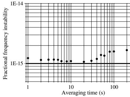
Fig. 5. Fractional frequency instability of one cavity-stabilized laser (dots). The solid line denotes the thermal-noise-limited frequency instability of approximate  $1 \times 10^{-15}$  for one cavity.
