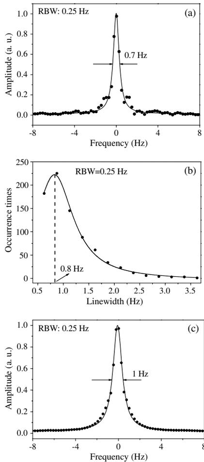
Fig. 3. Linewidth measurements when the RBW of the FFT spectrum analyzer is 0.25 Hz: (a) an example of the spectra of the beat note between two cavity-stabilized lasers (dots) and the Lorentzian fitting (solid curve), (b) linewidth distribution of approximately 800 groups of the spectra (dots) with 0.25 Hz step and the Lorentzian fitting (solid curve), and (c) an averaging spectrum of the beat note with center-overlapped (dots) and the Lorentzian fitting (solid curve).
