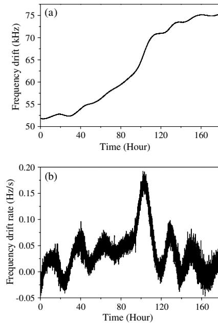
Fig. 4. (a) Relative frequency drift of the beat note between two cavity-stabilized lasers at 1064 nm over 7 days and (b) calculated relevant frequency drift rate.
