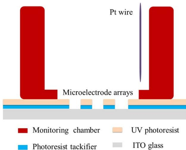
Fig. 1. Schematic diagram of the device for impedance monitoring.
