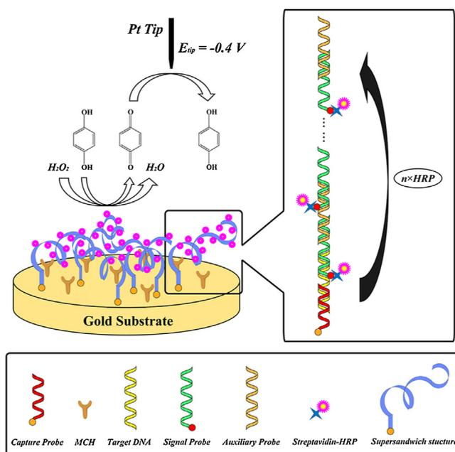
**Scheme 1.** Schematic of the fabrication and SECM detection of the proposed DNA biosensing platform.
