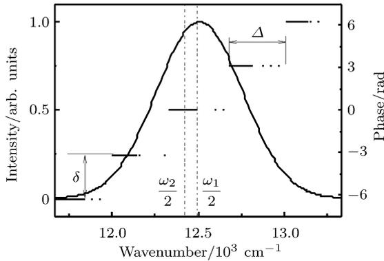
**Fig. 2.** Schematic diagram of the piecewise phase jump applied to the laser spectrum.  $\delta$  and  $\Delta$  represent the modulation amplitude and each segment spectral width, respectively. Here, each segment spectral width  $\Delta$  is set to be four times of  $\omega_1/2 - \omega_2/2$ .
