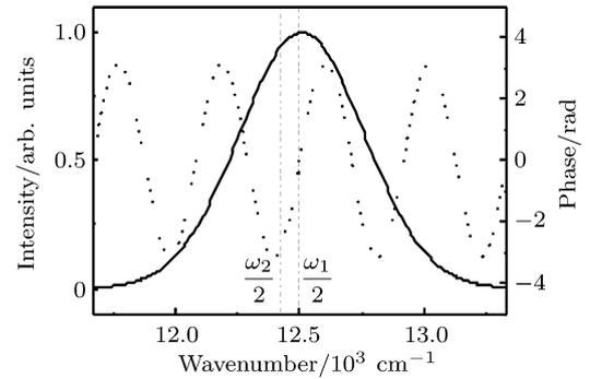
**Fig. 4.** The schematic diagram of the sinusoidal phase modulation ( $\Phi(\omega) = \alpha \sin[\beta(\omega - \omega_1/2)]$ ) applied to the laser spectrum, where  $\alpha$  is the amplitude of the phase modulation function, and  $\beta$  is the frequency of the sinusoidal oscillation.
