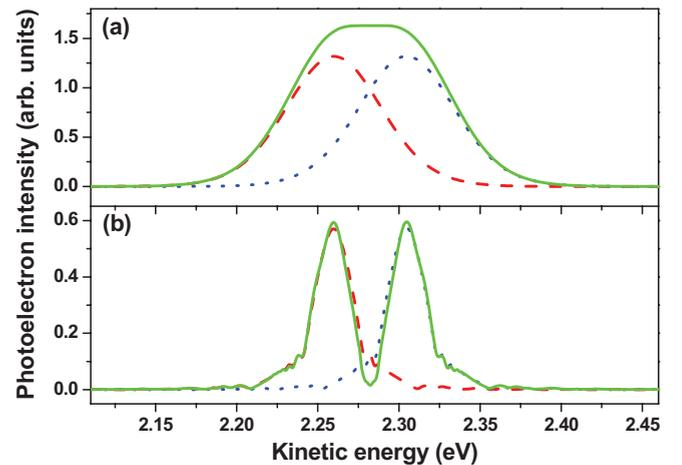
FIG. 3. (Color online) The (2+1) REMPI-PS (green solid lines) induced by (a) the transform-limited laser pulse and (b) the shaped laser pulse with modulation amplitude  $\alpha = 2 \times 10^5 \text{ fs}^3$  and phase step position  $\omega_{\text{step}} = 19955 \text{ cm}^{-1}$ , together with the contribution only from excited states  $8d$  (red dashed lines) and  $9d$  (blue dotted lines).
