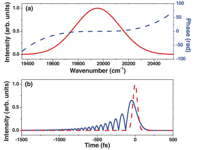
FIG. 2. (Color online) (a) The laser spectrum modulated by a cubic phase modulation. (b) The temporal intensity profile of the transform-limited laser pulse (red dashed line) and the shaped laser pulse by the cubic phase modulation with modulation amplitude  $\alpha = 5 \times 10^4 \text{ fs}^3$  and phase step position  $\omega_{\text{step}} = 19955 \text{ cm}^{-1}$  (blue solid line).
