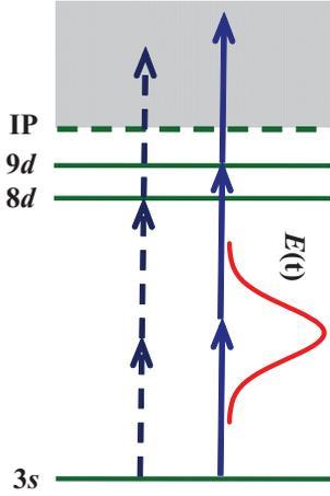
FIG. 1. (Color online) The schematic diagram of the (2+1) resonantly enhanced three-photon ionization process in a Na atom. The transition from ground state  $3s$  to excited state  $8d$  or  $9d$  is pumped by nonresonant two-photon absorption, and the populations in excited states  $8d$  and  $9d$  are ionized by single-photon absorption.
