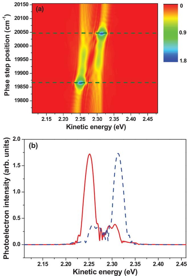
FIG. 4. (Color online) (a) The (2 + 1) REMPI-PS as a function of the phase step position  $\omega_{\text{step}}$  with modulation amplitude  $\alpha = 2 \times 10^5 \text{ fs}^3$ . (b) The (2 + 1) REMPI-PS for phase step position  $\omega_{\text{step}} = 19865$  (red solid line) and  $20045 \text{ cm}^{-1}$  (blue dashed line).
