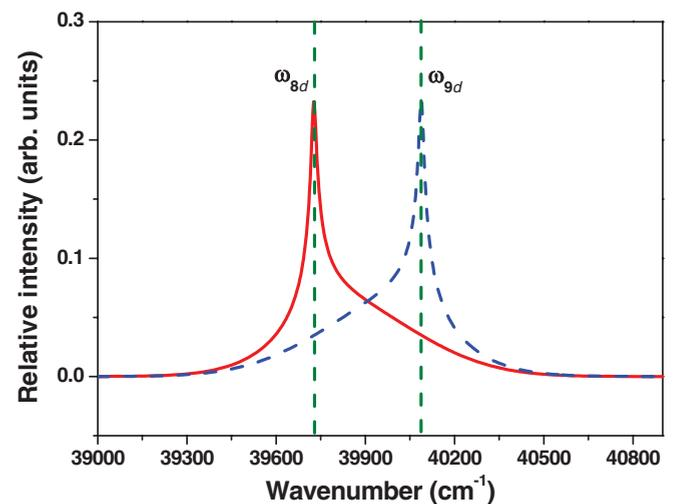
FIG. 6. (Color online) The two-photon power spectra of the shaped laser pulse with modulation  $\alpha = 2 \times 10^5 \text{ fs}^3$  for phase step position  $\omega_{\text{step}} = 19865$  (red solid line) and  $20045 \text{ cm}^{-1}$  (blue dashed line).
