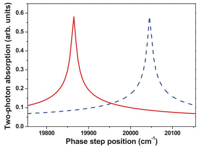
FIG. 5. (Color online) The two-photon transition probability in excited states  $8d$  and  $9d$ ,  $P_{8d}$  (red solid line) and  $P_{9d}$  (blue dashed line), as a function of the phase step position  $\omega_{\text{step}}$  with modulation amplitude  $\alpha = 2 \times 10^5 \text{ fs}^3$ .
