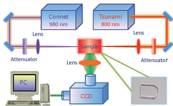
Fig. 1 The schematic diagram of the experimental arrangement for the two-color laser field excitation in the  $\text{Er}^{3+}/\text{Yb}^{3+}$ -codoped glass sample. Here, the glass sample picture is shown in the inset.
