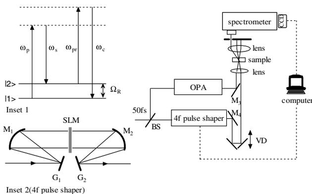
Fig. 1. The schematic diagram for experimental set-up (BS, beam-splitter; VD, variable delay line); Inset 1 is the schematic diagram for the CARS process; Inset 2 is the schematic diagram of 4 f pulse shaper composed of two grating ( $G_1$  and  $G_2$ ), spatial light modulator (SLM) and two con-focal concave mirrors ( $M_1$  and  $M_2$ ).
