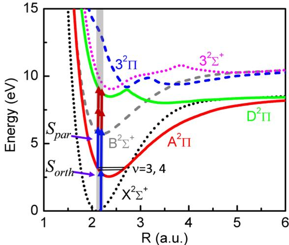
FIG. 5. The potential energy surfaces of involved electronic states of  $CO^+$  calculated by MOLPRO, where the Franck-Condon ionization region of the ground state CO is indicated by the grayed bar. The red (FW photon) and blue (SH photon) arrows indicate the transition pathways for the dissociation of  $CO^+$  with molecular axis parallel and orthogonal (labeled as  $S_{\text{par}}$  and  $S_{\text{orth}}$ ) to the polarization of the two-color field.
