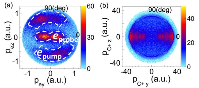
FIG. 2. Momentum distributions of (a) emitted electrons measured in coincidence with (b) C<sup>+</sup> fragments of the (C<sup>+</sup>, O) breakup channel.
