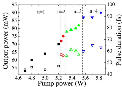
Fig. 6. The average output power (solid symbol) and the pulse duration (open symbol) as functions of the pump power, where  $n$  is the number of pulses in a round-trip time.
