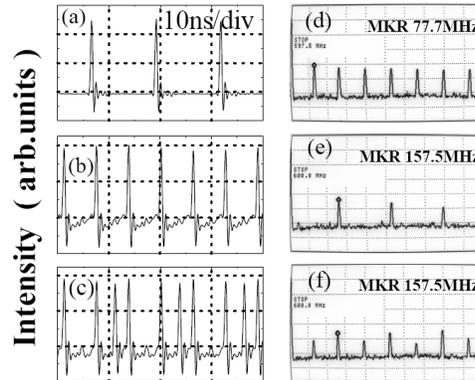
Fig. 3. Pulse trains and the corresponding rf-spectra observed while varying the position of Ti:S2. Normal mode locking (a and d), second harmonic mode-locking (b and e), and triple-pulse operation (c and f) are observed.
