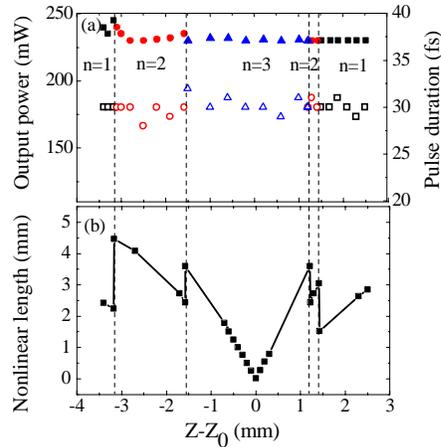
Fig. 2. (a) The average output power (solid symbol) and the pulse duration (open symbol) as functions of the position of Ti:S2 relative to the focus of the confocal cavity, where  $z$  is the position of Ti:S2 while  $z_0$  is the position of the focus, and  $n$  is the number of pulses in a round-trip time. (b) The effective nonlinear length as a function of the position.
