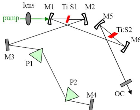
Fig. 1. Schematic of the Ti:Sapphire laser. Ti:S1 and Ti:S2 are two Ti:sapphire crystals with 2.5 mm and 5 mm thickness, respectively. M1-M6 are broadband HR coated chirped mirrors and OC is the output coupler. M1, M2, M5 and M6 are concave mirrors with a curvature radius of 100 mm. The fused silica prisms P1 and P2 supply tunable dispersion.
