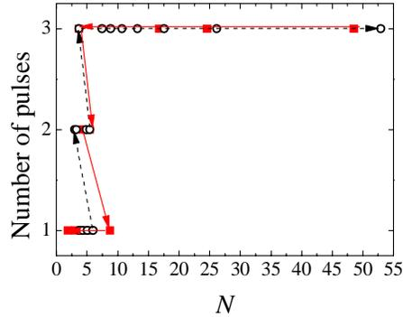
Fig. 5. The dependence of the number of pulses in a round-trip time on the value of  $N$ . The arrows show the pulse evolution while Ti:S2 is translated hereabout the confocal focus orderly. Here dash line and circle correspond to the situation that Ti:S2 moves towards the focus while solid line and square correspond to the opposite.
