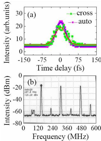
Fig. 4. (a). Cross-correlation (green line and symbol) and auto-correlation (magenta line and symbol) measurements when the laser is second harmonic mode-locked. The blue (red) line is the Gaussian simulation of the cross-correlation (auto-correlation) trace. (b) For the second harmonic mode-locking, the RF spectrum shows a super-mode suppression  $>38$  dB.
