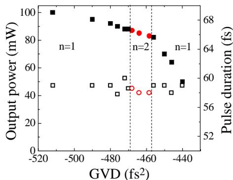
Fig. 7. The average output power (solid symbol) and pulse duration (open symbol) as functions of the net negative intra-cavity GVD where  $n$  is the number of pulses.
