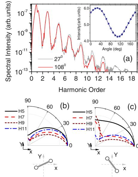
FIG. 2. (Color online) (a) The generated harmonic spectra from nonpolar molecules with SPR-enhanced optical fields. The inset is the conversion efficiency of the generated even-order harmonics as a function of the orientation angle of the nonpolar molecule. (b) and (c) plot the emission probabilities of the generated harmonics as a function of emission angle when the nonpolar molecule is oriented at angles of  $27^\circ$  and  $108^\circ$  relative to the surface, respectively.
