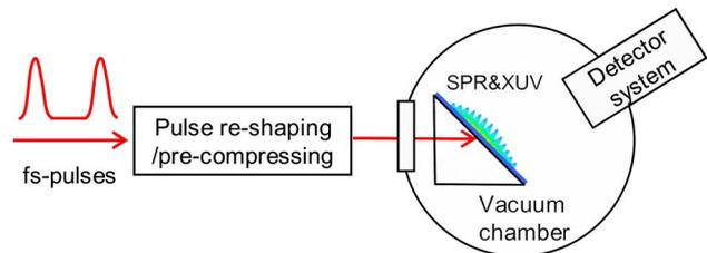
FIG. 1. (Color online) Schematic configuration of xuv frequency comb generation based on SPR-enhanced optical fields, where the incident fs pulses from the oscillator are prechirped or reshaped to manipulate the output spectra.
