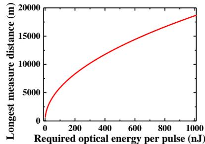
Fig. 4. The theoretical curve of output optical energy vs. largest measure distance.
