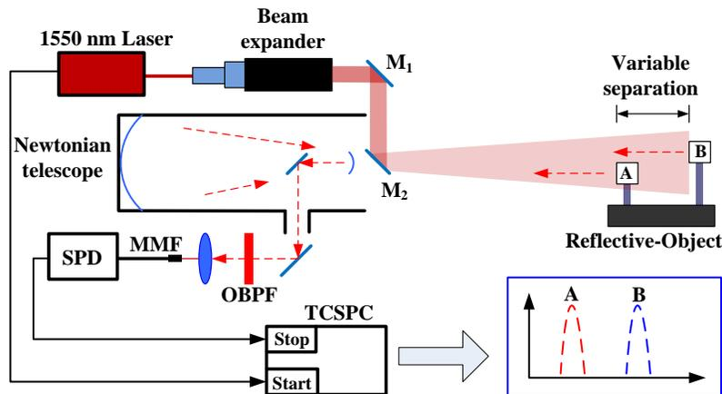
Fig. 1. Experimental setup of the laser ranging system based on single-photon detection at 1550 nm. SPD: single-photon detector based on InGaAs/InP APD; OBPF: optical bandpass filter (center wavelength: 1550.10 nm, FWHM: 6.47 nm); M1, M2: high-reflection mirrors; MMF: multimode fiber; TCSPC: time-correlated single-photon counting system (PicoHarp300, PicoQuant GmbH, Germany).
