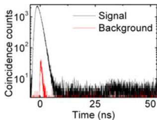
Fig. 7. Coincidence measurement between the pump pulses and SFG photons as well as the background counts.
