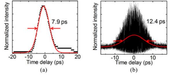
Fig. 3. Autocorrelation pulse profiles of (a) the signal source and (b) the pump source, respectively. Solid symbols in black are the experimental data and solid curves in red are the Gaussian fits to the data.
