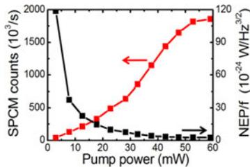
Fig. 6. Signal counts recorded by the Si-APD SPCM and NEP divided by the repetition rate as a function of the pump power.
