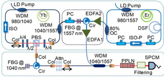
Fig. 1. Experimental setup of the synchronization pumping system. LD: laser diode; Cir: circulator; Col: collimator; PC: polarization controller; DSF: dispersion-shifted fiber; OC: output coupler; ISO: optical isolator; ISO-P: polarization-dependent isolator; PBS: polarization beam splitter; Attn: attenuator; and SPCM: single-photon counting module.
