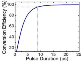
Fig. 4. Simulated conversion efficiency as a function of the pump pulse duration by assuming a Gaussian signal pulse with the FWHM of 5.6 ps. The hollow circle shows the experimental situation.
