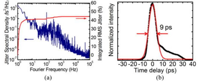
Fig. 5. (a) Timing jitter power spectral density (left) and the integrated timing jitter in Fourier domain (right). (b) Cross-correlation trace of the synchronized lasers. Solid symbols in black are the experimental data and solid curve in red is the Gaussian fit to the data.
