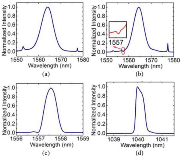
Fig. 2. (a) Er-doped fiber laser spectrum. (b) Spectrum of the FBG transmission. Inset: zoomed spectrum around 1557 nm. (c) Spectrum of the FBG reflection. (d) Spectrum of the signal source from the Yb-doped fiber laser.
