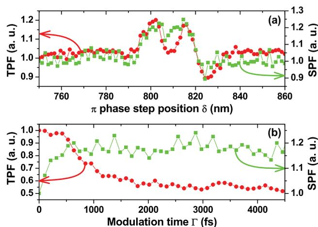
FIG. 4. The normalized SPF (green squares) and TPF (red circles) intensities as the function of the step position  $\delta$  of the  $\pi$  phase modulation (a) and the modulation time  $\Gamma$  of the square phase modulation (b) with the higher laser intensity of  $1.2 \times 10^{13} \text{ W/cm}^2$ .
