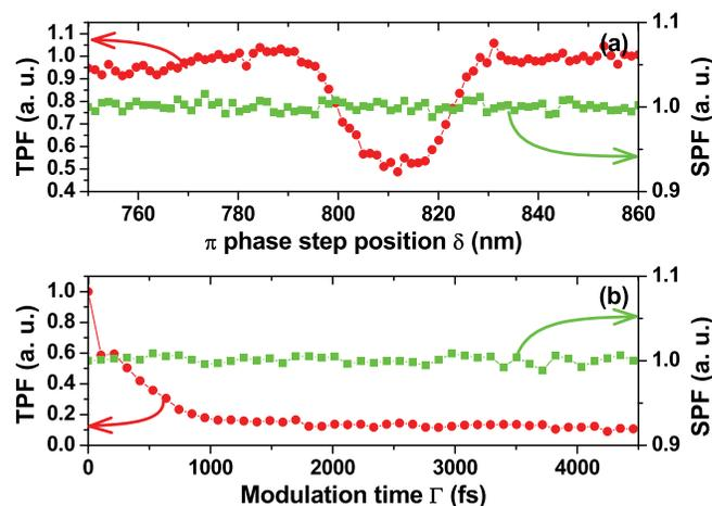
FIG. 3. The normalized SPF (green squares) and TPF (red circles) intensities as the function of the step position  $\delta$  of the  $\pi$  phase modulation (a) and the modulation time  $\Gamma$  of the square phase modulation (b) with the lower laser intensity of  $8.4 \times 10^{10}\text{ W/cm}^2$ .
