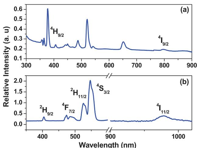
FIG. 2. The absorption (a) and fluorescence spectra (b) of the glass sample  $60\text{SiO}_2\text{-}20\text{Al}_2\text{O}_3\text{-}20\text{CaF}_2$  doped with  $\text{Er}^{3+}$  ions.
