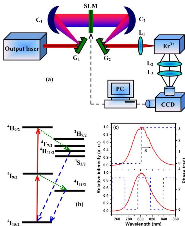
FIG. 1. (a) Schematic diagram of the experimental arrangement. The output femtosecond laser pulse is shaped by a 4f-configuration pulse shaping system. (b) Energy level diagram of the single and two-photon absorption and fluorescence detected schemes in the glass sample 60SiO<sub>2</sub>-20Al<sub>2</sub>O<sub>3</sub>-20CaF<sub>2</sub> doped with Er<sup>3+</sup> ions. (c) The laser spectrum is modulated by a  $\pi$  (upper panel) or square (lower panel) phase modulation.
