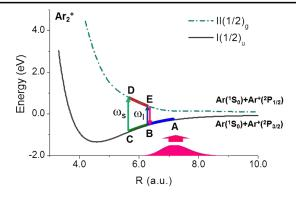
FIG. 1 (color online). Sketch of the  ${\rm Ar_2}^+$  dissociation dynamics in two mutually delayed and detuned ultrashort laser pulses with central frequencies  $\omega_s$  and  $\omega_l$  that allow resonant one-photon transitions at internuclear distances R indicated by C, D and B, E, respectively. The red profile shows the nuclear probability density of the  ${\rm Ar_2}$  ground state.
