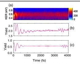
FIG. 4 (color online). (a) Measured time-dependent KER spectrum as in Fig. 3(a), but for an increased pump-pulse peak intensity of  $9 \times 10^{14} \text{ W/cm}^2$  and an extended delay range. (b) Dissociation yield obtained by integration over the KER range in (a). (c) The calculated dissociation yield for the same KER range.
